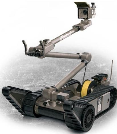
Figure 4. The iRobot 510 PackBot® for explosive ordnance disposal (iRobot, 2015).
