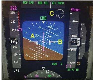
**Fig. 1.** The display on the B737-800's primary flight display
